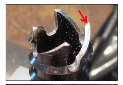
File down until the flat spot is gone and a new edge is formed on the leading side of the tooth.
