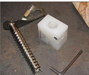
Another option is to make a block from a piece of plastic with a pinch bolt for securing the screw.
