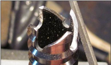
With the flat side of the file remove any burrs along the outer edge of the tooth.
