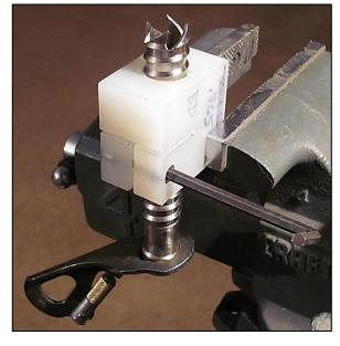
The advantage of this method is that the block can remain clamped in the vise while the screw is repositioned by tightening/loosening the pinch bolt.
